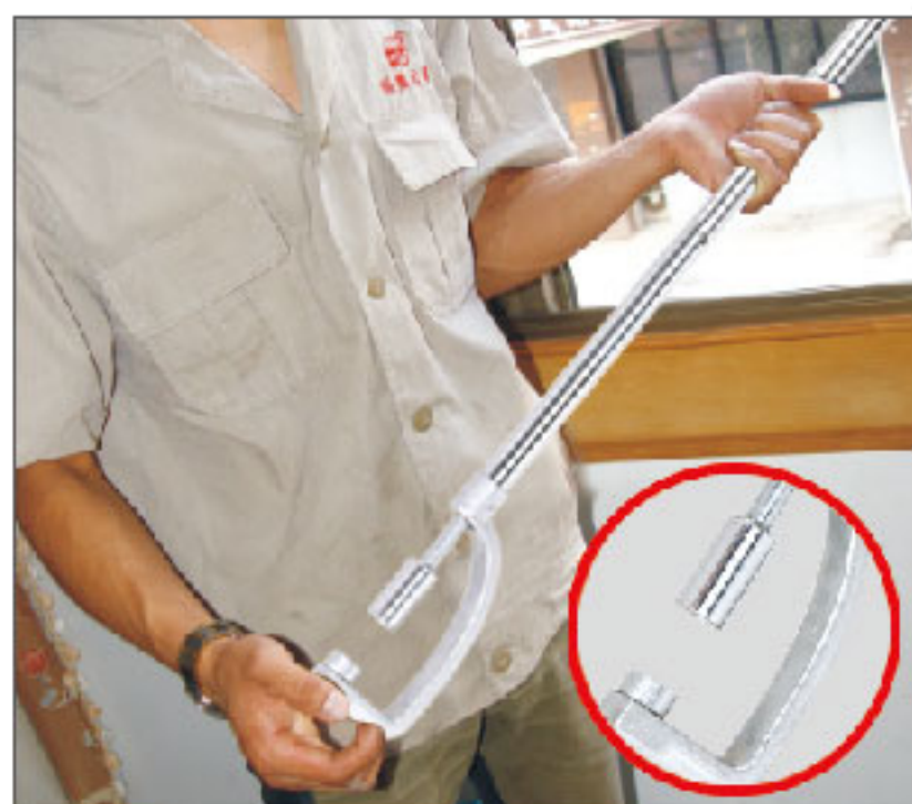
Put screw in spanner 强磁吸住螺丝
